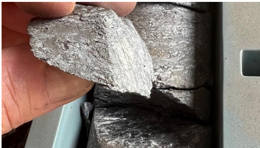
Figure 3: Graphitic Schist from LEDD_3 at 18.5m (interval 18-19m assayed 11.3% TGC)
